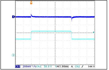
Figure 6: Output voltage response to step-change in input voltage (1000 V/ms). Load cap: 100 µF, electrolytic output capacitance. Ch 1: Vout (200 mV/div), Ch 2: Vin (50 V/div).
