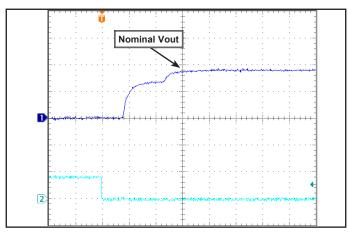
**Common Figure 1: Startup Waveform** (typical), input voltage pre-applied, ON/ OFF Pin on Ch 2.
