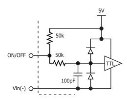
Figure B: Internal ON/OFF pin circuitry
