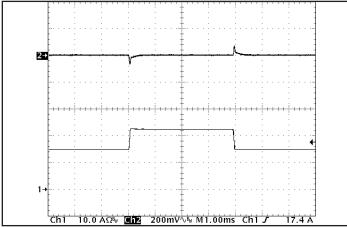
Figure 5: Output voltage response to step-change in load current (66 %-100 %-66 % of Iout(max);  $dI/dt = 0.1 A/\mu s$ ). Load cap: 15  $\mu F$  tantalum cap and 1  $\mu F$  ceramic cap. Ch 1: Iout (10 A/div), Ch 2: Iout (200 Iout).
